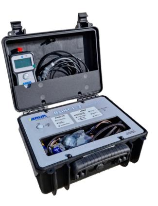
BUKCI-3 connects to live LV Cable at 115V, 230V, or 400V; the transmitter will automatically configure to the connected power.
