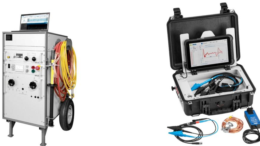
*The IRG 400 time domain reflectometer in the built-in version for a 19" rack (1 RU) and in the portable case version with removable tablet. (Pictures: BAUR GmbH)*
